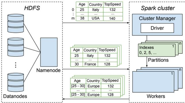
Fig. 2. Architecture and working of the distributed anonymization system
