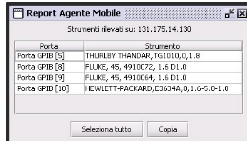
Fig. 6 – An example of an implemented Mobile Agent which is able to recognize the instruments connected by IEEE 488 to the PC.
